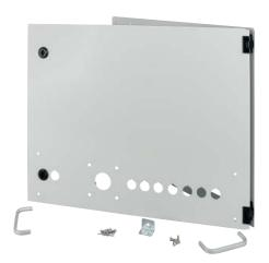
With a metal thickness of 2mm at both the front plate and the support plate, the steel front plate provides maximum stability. Both parts are available with a RAL7035 coated structure (on request also in a special colour) with an IP31 and IP55 degree of protection, and are provided with right-hand hinges.
