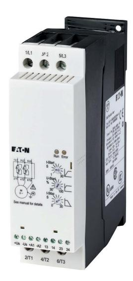
AC motors are used as the ideal drive in various industrial and commercial machines. In many cases, however, direct starting or star-delta starting is not always the best choice. At least then it is time for soft starters to be used. With soft starters you do not have high starting currents or an abrupt insertion of full torque, but you can properly ramp up time, inrush current and torque.
