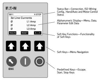
The Status Bar at the top of the display indicates the operating and communicating status of the S811+ and DIM.
