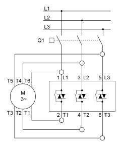
**Note:** For soft starters used in an Inside-the-Delta application, use of a shunt trip breaker is highly recommended. The S811+ may be configured to actuate a shunt trip breaker on user selected Fault Trip parameters.
