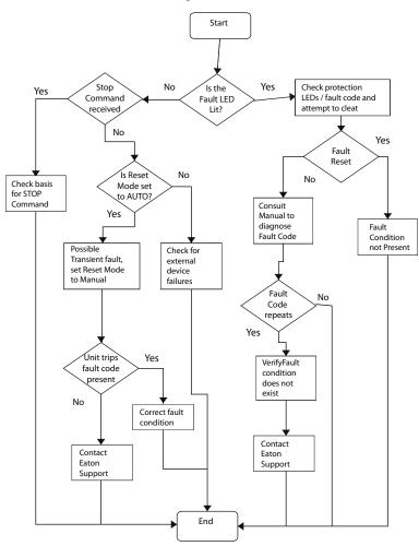
In extreme cases, it may be necessary to reset parameter settings and operating values to restore proper operation. The S811+ may be reset by following the instruction below.
