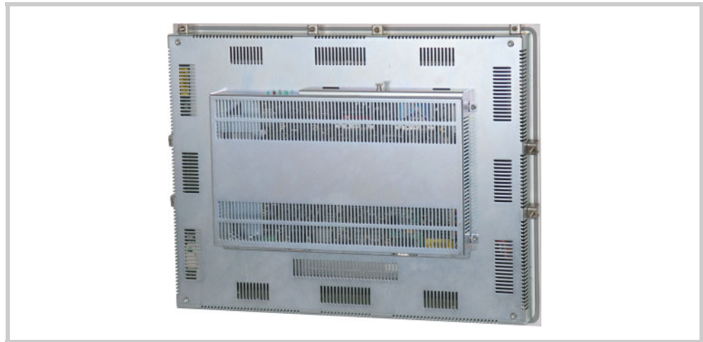
Fig. 27 15" devices with twelve retaining brackets (meet IP65 requirements)
