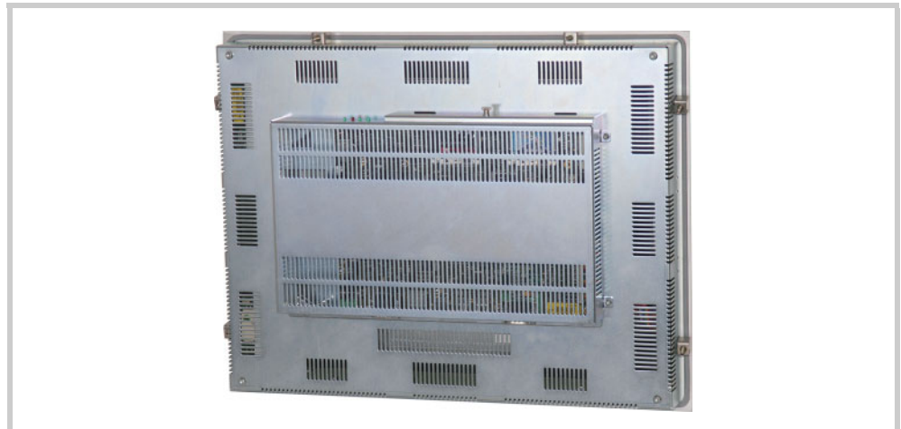
Fig. 26 15" devices with eight retaining brackets (do not meet IP65 requirements)
