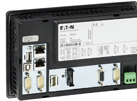
Figure 4: Service side with optional interfaces XV-303-70-CE2-A00-1C
