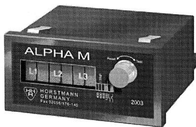
The indicator unit contains the electronic circuit, a miniature generator with turning knob, and three rectangular flags. The indication persists until it is reset by hand by rapidly turning the turning knob to the left.
