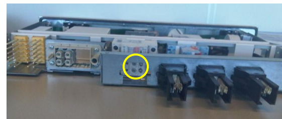
Fig. 3-11 Earth Fault Relay settings adjustment (1)
