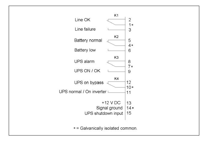
**Table 1.** *UPS Alarm/OK* and *Bypass* relay informations are not supported by the Powerware 5125 and Powerware 9125 UPSes.
