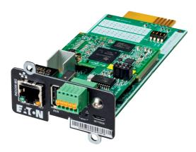
Industrial Gateway Card is compatible with the MODBUS communications protocol.
