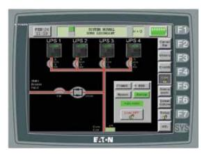
The 9395 SBM features a colour LCD touch screen that allows monitoring of the entire UPS system as a whole and the statuses of individual UPSs.
